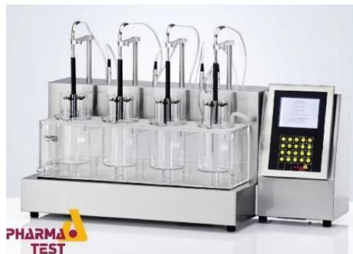
**Gambar 5.2. Disintegration Tester**
